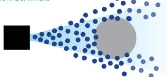
The Victory Series provide a fast and efficient application of chemicals. When the charged particles reach the desired surface, they uniformly disperse the product. The particles subsequently maintain their cationic charges for approximately 2 to 3 seconds – thus preventing grouting. This allows the solution to cover hidden and shaded areas, and also allows the user to cover a large area in a limited time.
